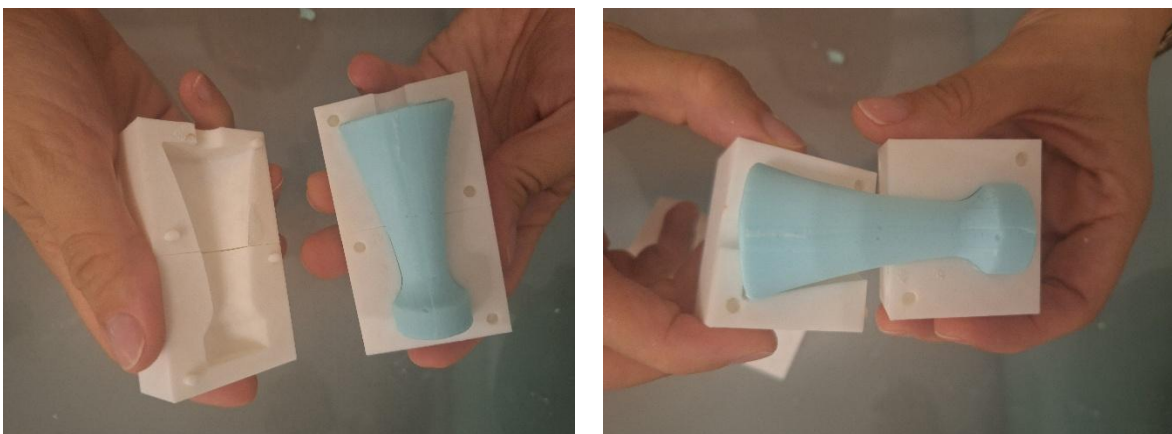
Figure 85. Unmoulding the finished soap chess pieces from two (left) and four-piece moulds (right).
