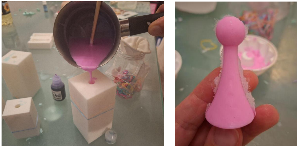
Figure 82. Casting the soap into tightly sealed moulds.
