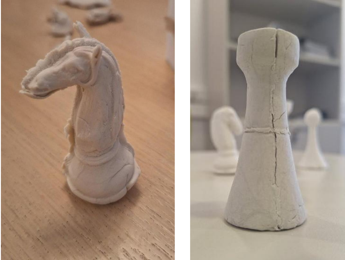
Figure 76. Left: A chariot piece made of plasticine. The seams due to excess material are clearly visible. Right: Using liquid clay and the mould. After drying, the clay presents cracks.
