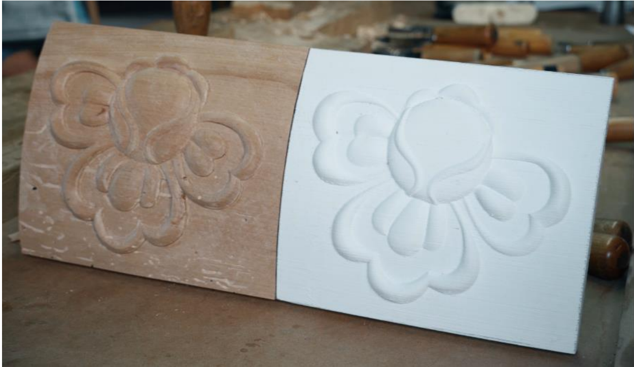
Figure 79. Comparison between the final wood-carved piece and the 3D printed piece. CETEM (2025) / CETEM
