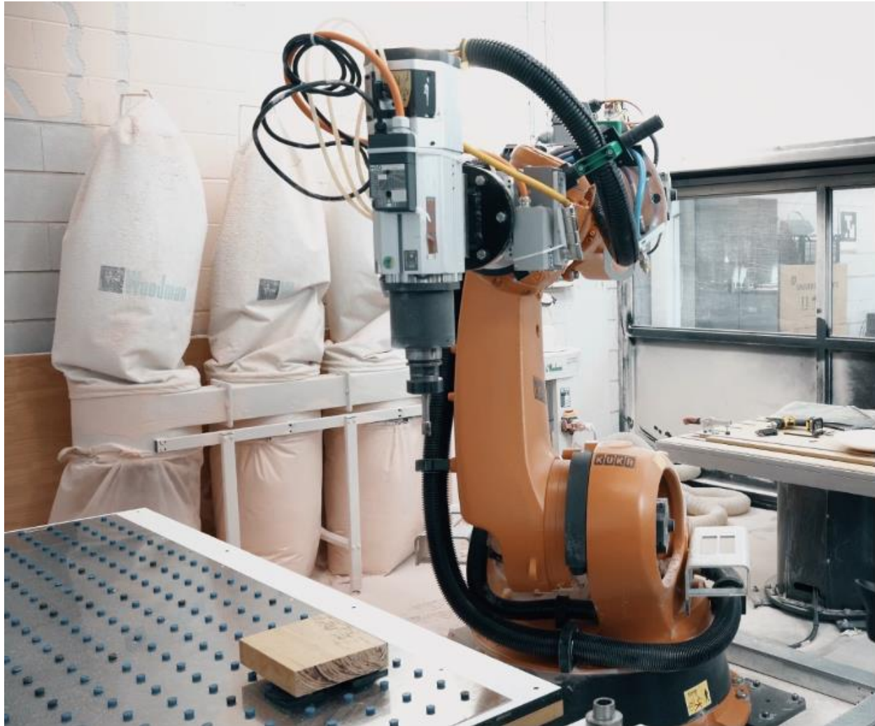
Figure 73. Anthropomorphic robot used as a CNC machine for preparing and curving the wood piece, CETEM (2025) / CETEM
