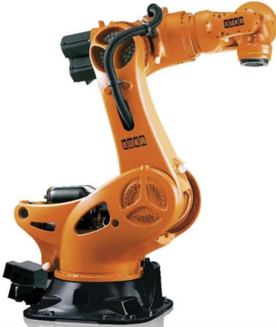
Figure 81. A KUKA anthropomorphic robot used as a CNC machine. CETEM (2025) / CETEM
