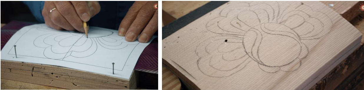
Figure 77. Woodcarver Francisco Sánchez transfers patterns from paper to the wooden piece / CETEM.
