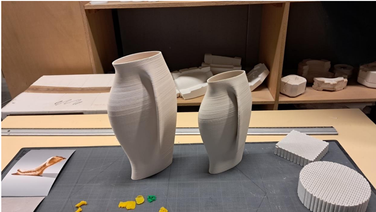
Figure 20. Examples of 3D printed ceramic pieces, Plaster Simulator Workshop, ENSAD Limoges, CCE Research
