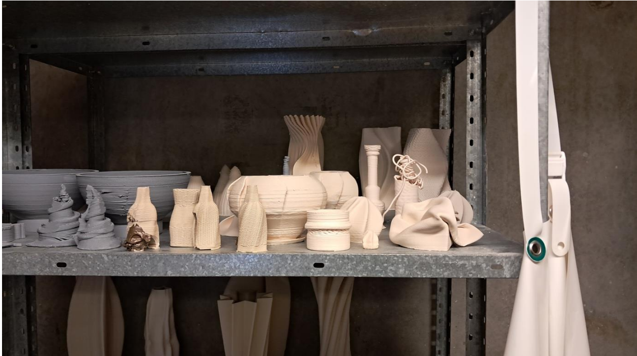
Figure 23. Ceramic 3D printed pieces, Plaster Simulator Workshop, CCE Laboratory, ENSAD Limoges (2025) © Inés Moreno/CNAM
