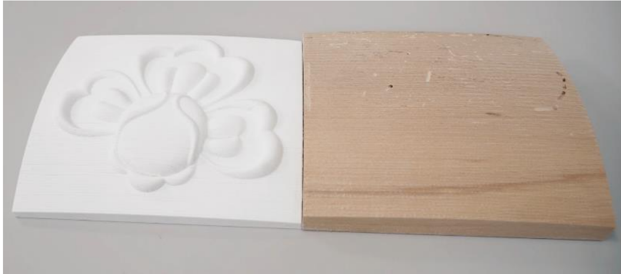
Figure 75. Comparison between the printed model and the prepared wood for woodcarving. CETEM (2025) / CETEM
