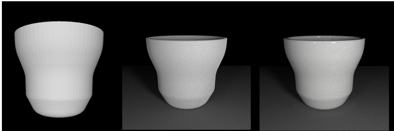
Figure 5. Comparison between (left) a MeshLab shaded viewport preview (using surface normals for smooth appearance) and (right) a neutral physically based render (single white point light). PBR rendering provides physically consistent shading cues, highlights, and shadow structures, which more effectively convey perceived 3D form and curvature for design review.
