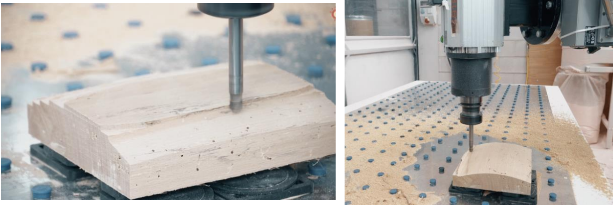
Figure 74. CAD model of the wood piece. The CNC robot is working. CETEM (2025) / CETEM
