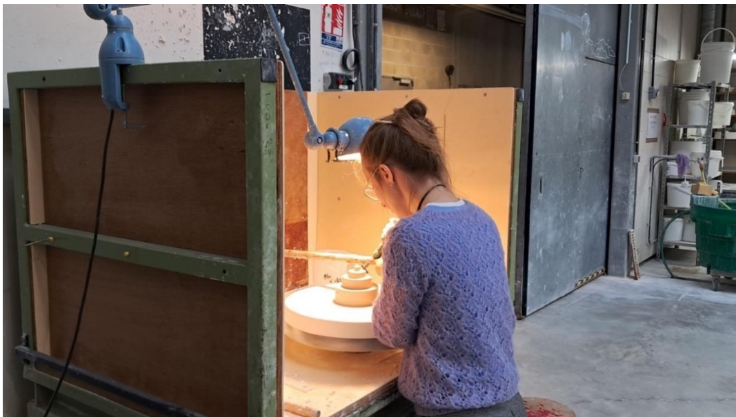
Figure 90 - Plaster Wheel turning process during the Simulator Workshop at the Porcelain Workshop, ENSAD Limoges - © Inés Moreno / Cnam
