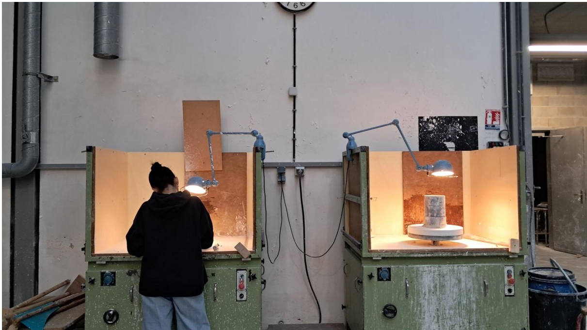
Figure 92 - Plaster Wheel turning process during the Simulator Workshop at the Porcelain Workshop, ENSAD Limoges © Inés Moreno / Cnam
