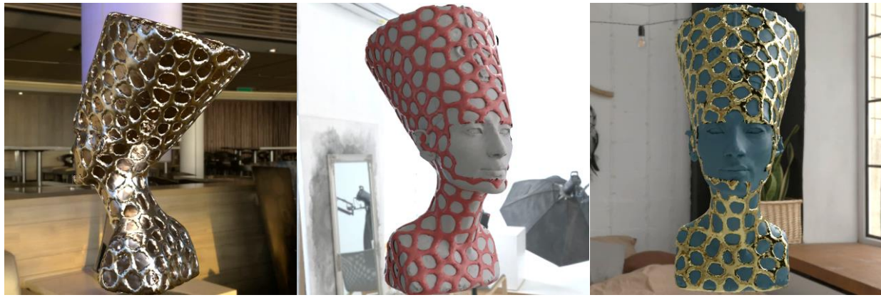
Figure 14. Multi-material preview of a two-part (interlocking) sculpture: renderings from multiple viewpoints showing distinct material assignments per part.
