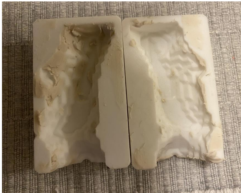
Figure 34. A two-part mould.
