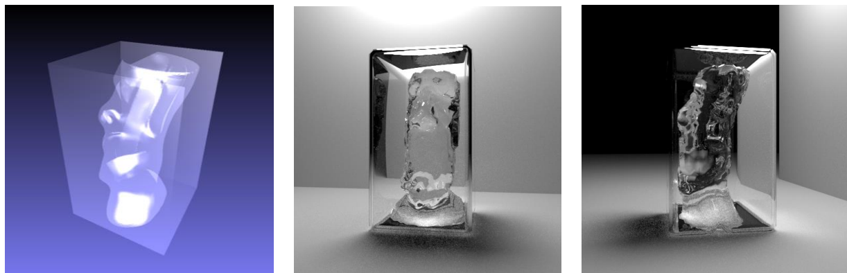
Figure 32. Rendering of the mould 3D model using transparency to illustrate its hollow structure.
