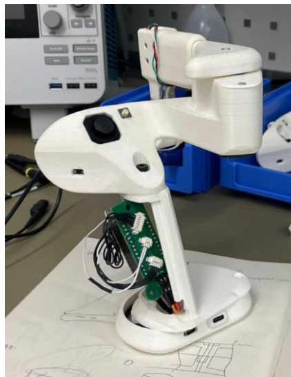
Figure: The electronics components are combined in the handle of the controller for easy access and assembly. This also establishes the center of gravity and leads to a comfortable experience holding, moving, and operating the controller.
