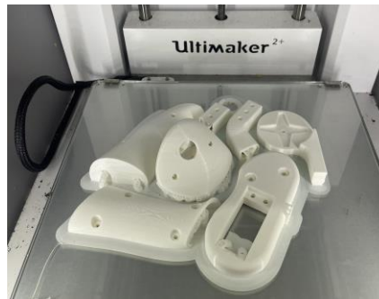
Figure: The individual parts of the controller are 3D printed from various materials to ensure sturdiness during operation, limited amounts of wear during use, and replicability in case of needed maintenance.
