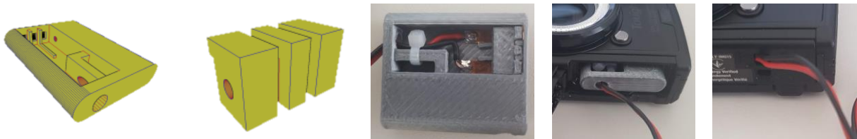
Figure 56. Designs of a battery emulator and photographs of its implementation.
