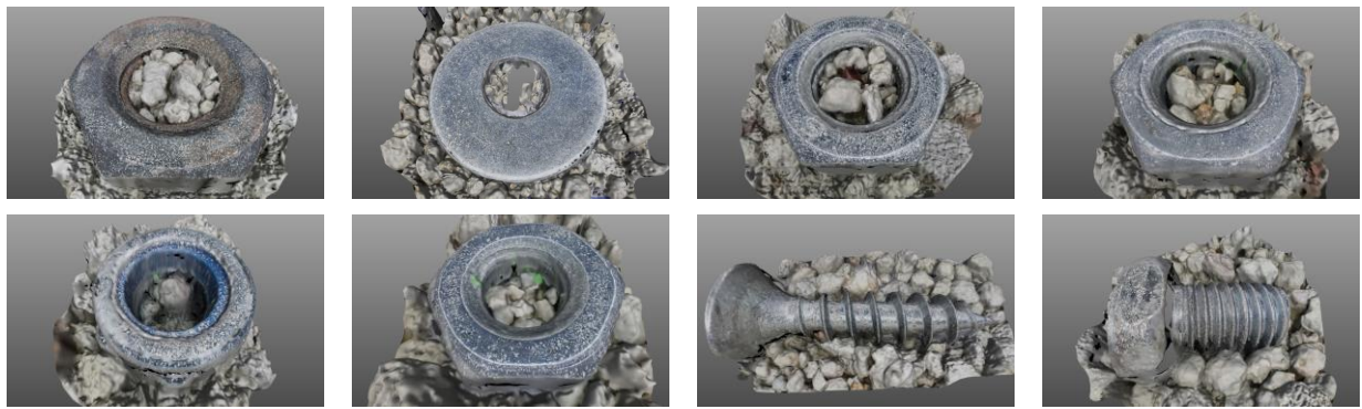
Figure 23. Textured renderings of the obtained reconstructions of the metallic nuts and screws.
