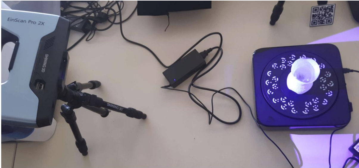
Figure 32. A static structured-light experimental setup used for the acquisition of the reference 3D reconstructions.
