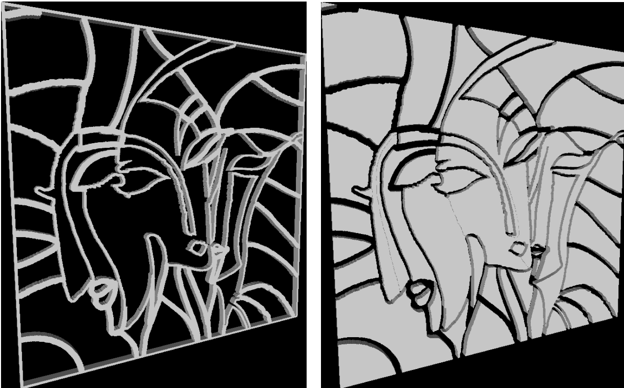
Figure 83. 3D model of a came framework (left) and its glass pieces (right).
