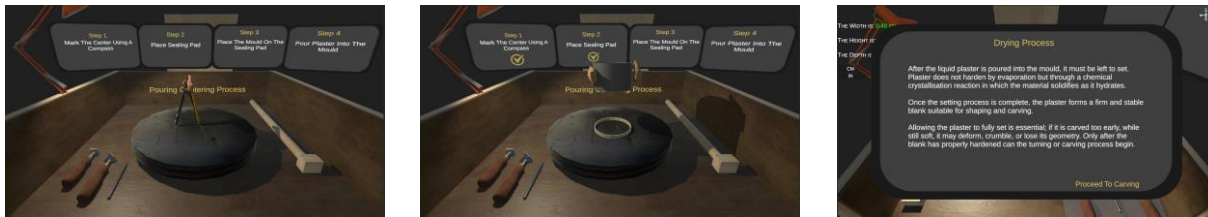
Figure 109. Version 5. Scene A (Preparation). Left: Compass-based centre marking of the model. Centre: Sealing pad placement between the model and mould. Right: Information display accompanying the animated drying process.
