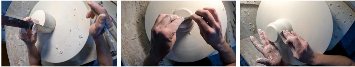
Figure 96. Egocentric views from straightness and dimensional verification (left), planing with a handheld metal strip (centre), and surface finishing with an abrasive pad (right).
