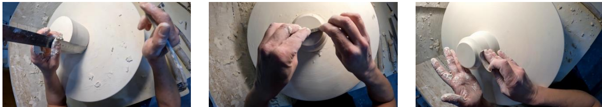
Figure 97. Egocentric views from straightness and dimensional verification (left), planing with a handheld metal strip (centre), and surface finishing with an abrasive pad (right).
