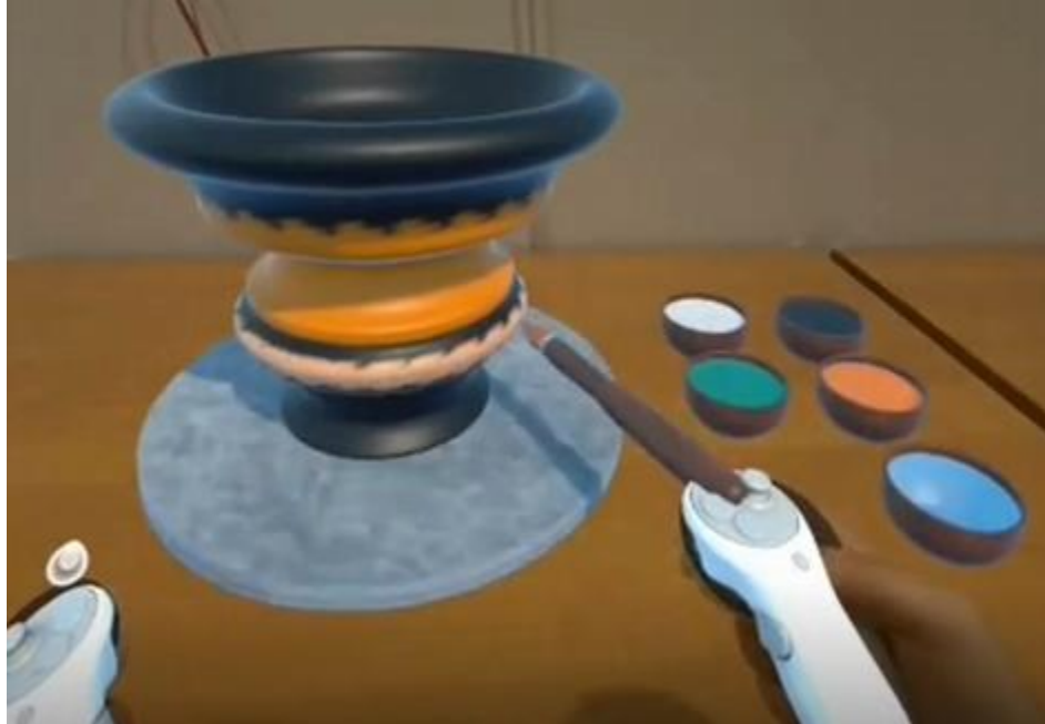
Figure 57. Decoration as an independent appearance layer. Painting updates per-vertex colour attributes on the already-generated vessel mesh; the solids-by-revolution geometry remains unchanged during finishing. A water jar clears the brush and erases colour to support rapid correction during practice.
