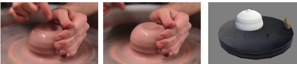
Figure 98. Centring in clay pottery versus plaster turning. Stills from a clay pottery documentary illustrate hand-based centring through pushing of the plastic clay body, where the stabilising hand provides feedback (left, middle). Rejected prototype implementing pottery-style centring (right). The prototype modelled centring as a hand-driven force interaction that attempts to push the rotating workpiece into alignment.
