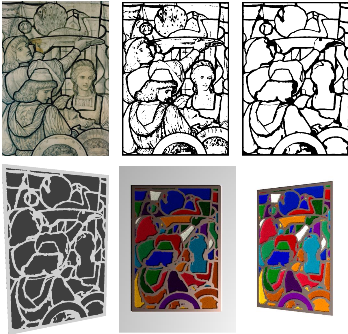
Figure 79. Validation of intrusion repair on a historical cartoon design. (Left) Source cartoon (Bosdet) used as input. (Middle-left) Extracted piece boundaries showing sharp inward intrusions that would yield fragile glass points. (Middle-right) Intrusion repair by constrained bridging of the intrusion border points, removing the high-curvature cusp while preserving the surrounding contour. (Right) Resulting validated 3D assembly (glass tiles + recomputed came), rendered with the Craeft PBR toolbox to preview the visual outcome under physically based light transport.
