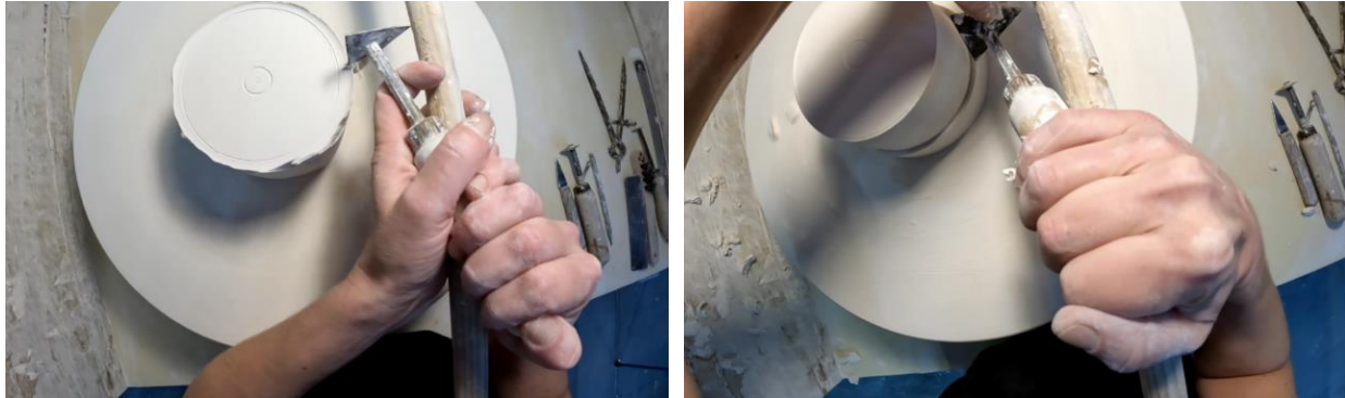
Figure 94. Egocentric views demonstrating the use of handheld turning tools, cutting the plaster workpiece.
