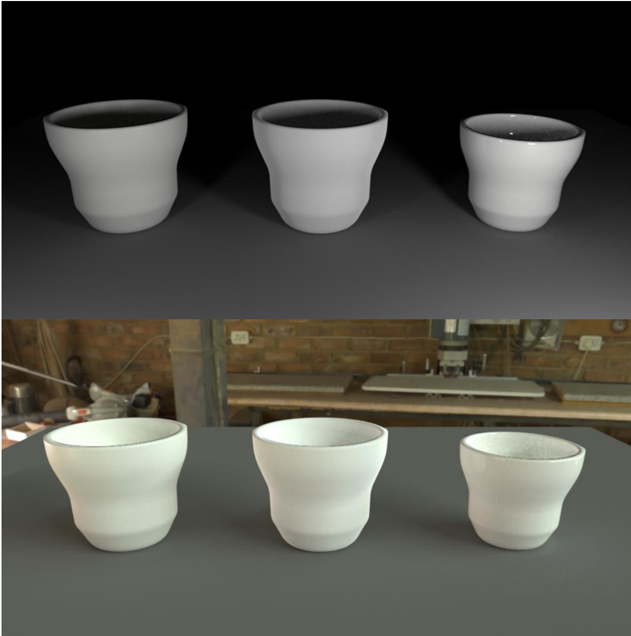
Figure 111. Physically based rendering (PBR) of a porcelain cup, comparing simulated material properties and geometric shrinkage. Left: The plaster master exhibits a satin finish. Centre: The calcined plaster master shows a characteristic matte, chalky surface. Right: The fired porcelain piece demonstrates a 14% volumetric shrinkage and a high-gloss glaze. Renders were generated simulating indicative studio lighting (top) and workshop illumination (bottom).
