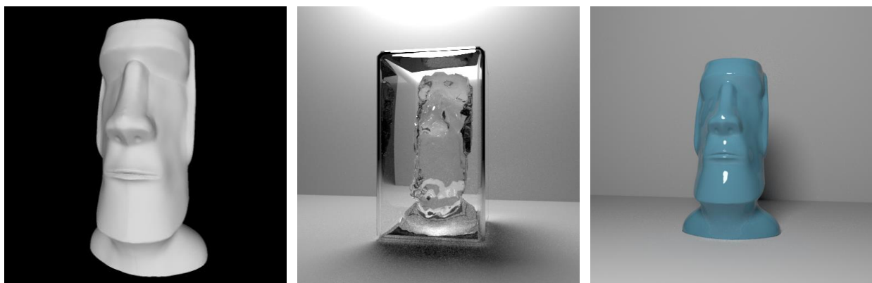
Figure 62. Left: Original model. Middle: Visualisation of the corresponding mould as transparent. Right: Predicted cast. This middle visualisation is animated in https://youtu.be/MFrC8m9ddCU to demonstrate the quality of the mesh created using the marching cubes algorithm.
