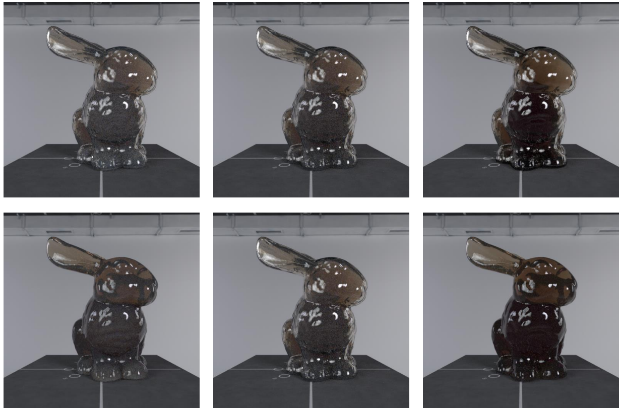
Figure 40. Effect of bulk-scattering anisotropy on glass appearance (solid vs hollow). Top row: hollow 2.5 mm shell; bottom row: solid. Left to right: g = -0.5 (backwards-biased), g = 0.0 (isotropic), g = 0.5 (forward-biased). Geometry, illumination, and interface finish are held constant to isolate the perceptual impact of bulk scattering.
