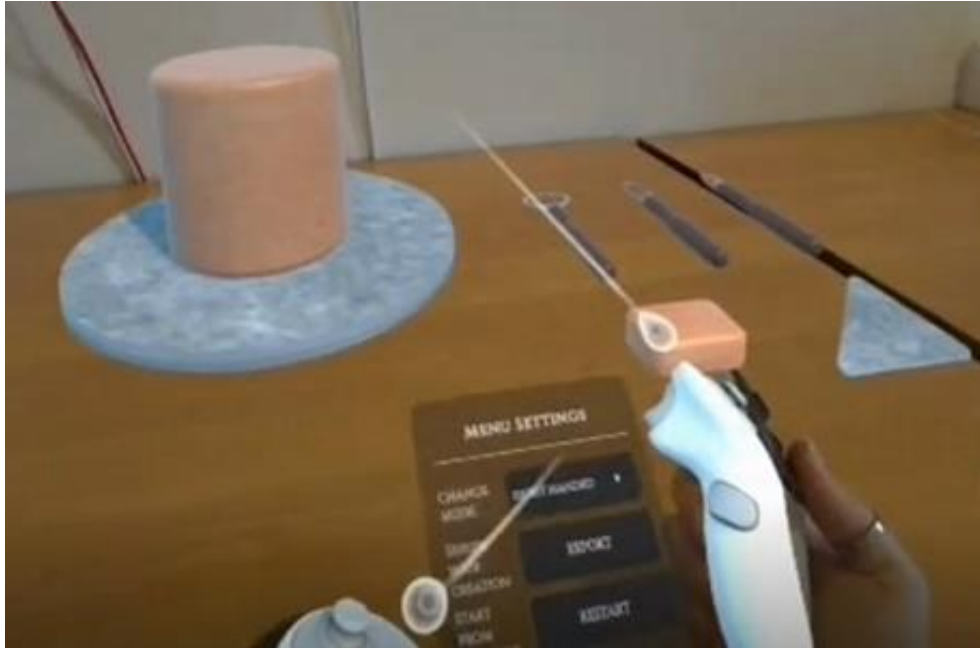
Figure 55. Unity/XR integration of the solids-by-revolution pottery module (workspace overview). In-headset workspace showing (1) wrist system menu, (2) the authoritative clay mesh, (3) the base/wheel controller that governs rotation state, and (4) pottery tools for shaping and decoration. The Unity layer drives interaction and feedback, while the underlying generator/API maintains the vessel geometry.
