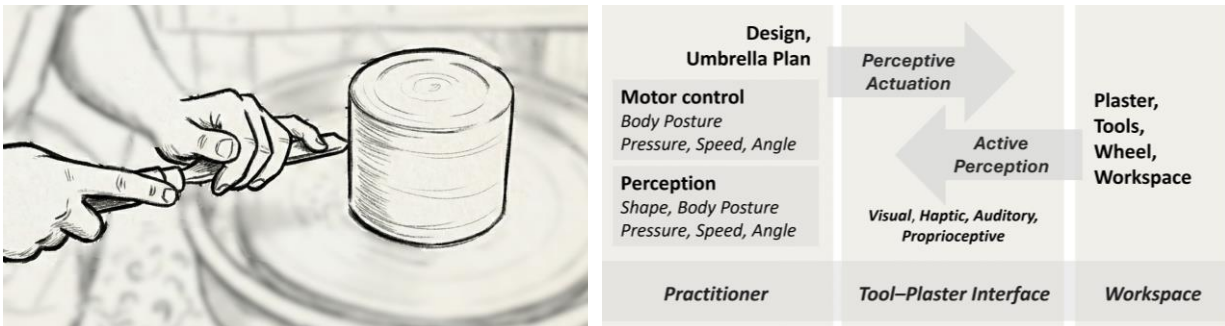
Figure 91. A practitioner engaged in plaster turning (left). The diagram (right) illustrates the continuous feedback loop, where the maker modulates tool actuation in real-time response to sensory cues.
