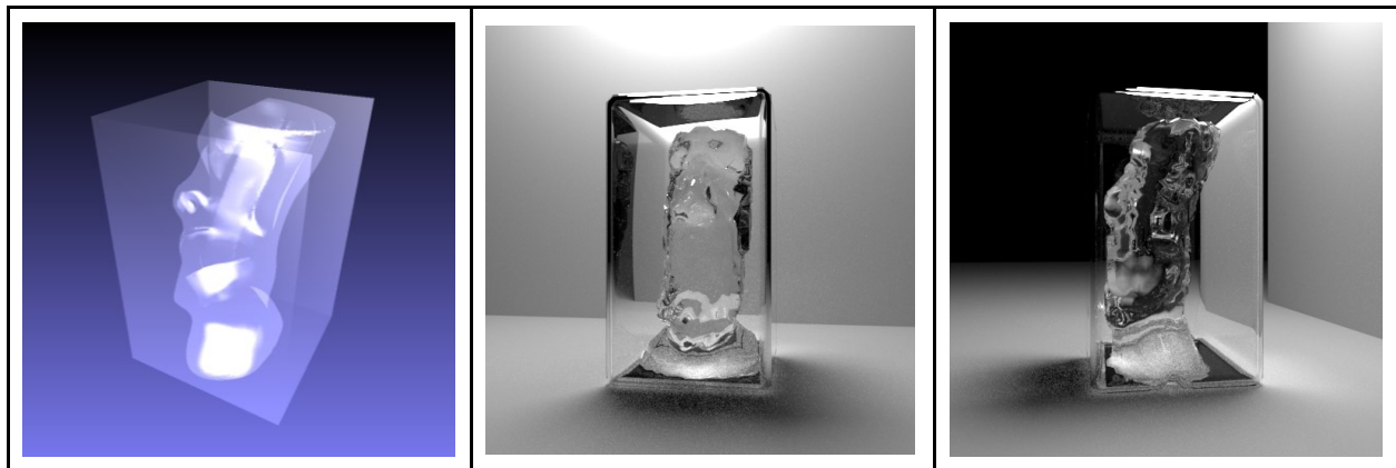
Figure 22. Rendering of the mould 3D model using transparency to illustrate its hollow structure.
